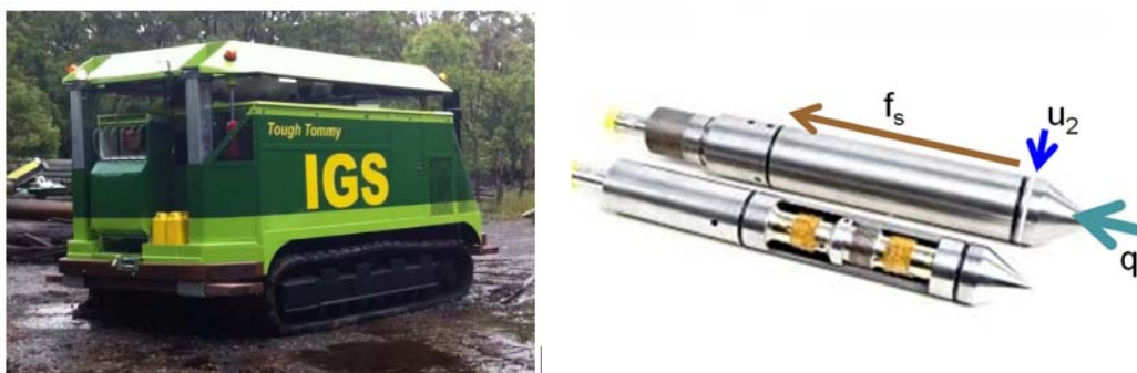
Figure 4-1: Illustration of CPT rig (left) and probe details (right)
