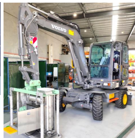
Robotic blasthole measurement
