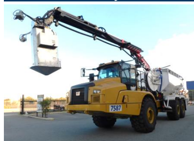
Robotic explosive placement
