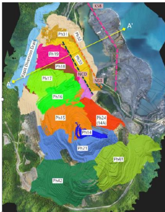
Figure 4.6 Lihir pit phases plan view
