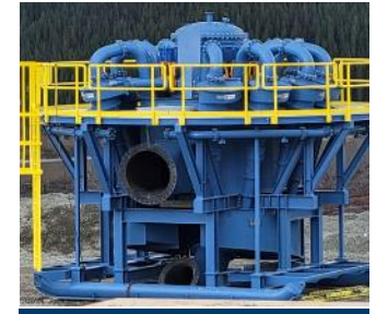
Cyclone sand construction for TIA enabled with commissioning of Cyclopac
