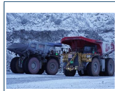
Rebuilt 793F truck fleet with 'Right Weight Body' trays. Higher capacity with improved operator comfort cabins
